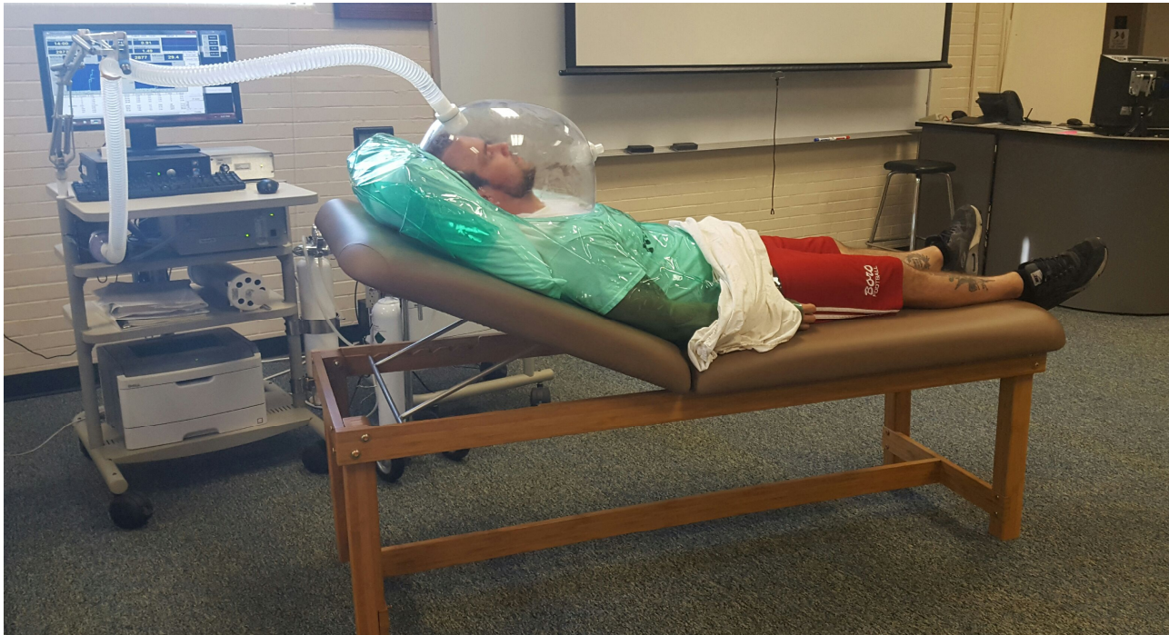
Figure 1. Experimental Set-up Using Ventilating Hood Technique.
