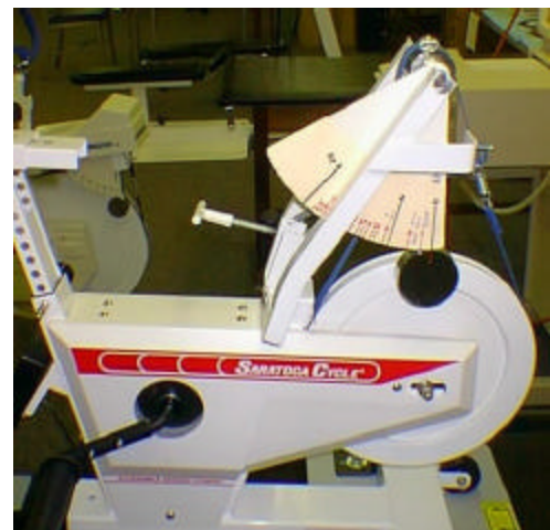
Figure 1. Saratoga Cycle ergometer modified with a Monark 818 tension mechanism. The faceplate was recalibrated for this device.
