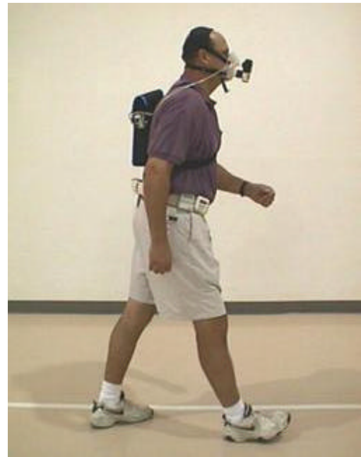
Figure 1. Photograph of a subject performing the walk test wearing the AeroSport KB1-C unit harnessed to his back and with the Caltrac and BioTrainer accelerometers clipped to a belt around the subject's waist.
